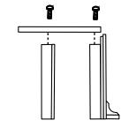
Tap all carriage bolts on top of head with hammer to seat square into wood, at this point only finger tighten flange nuts.
