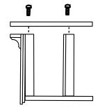
**4.** Set upright attach (2) top shelf vertical supports to main structure with 2" bolts and flange nuts.
